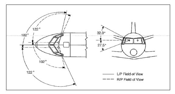
Figure 3 External vision angles from Saab pilots' seats (Source: Saab SF340A aircraft operations manual.)
