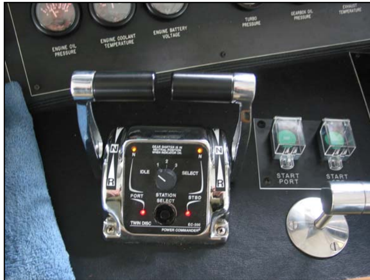
Figure 5 EC 200 main controller with illuminated station select and neutral lights
