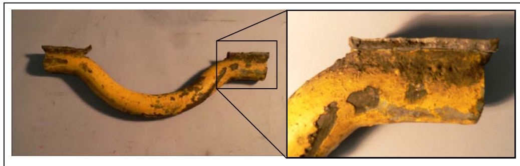
Figure 15 Truck lashing point, magnified end showing failure of base metal below the weld
