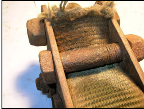
Figure 19 Location of failure in brown broken strop “A”
