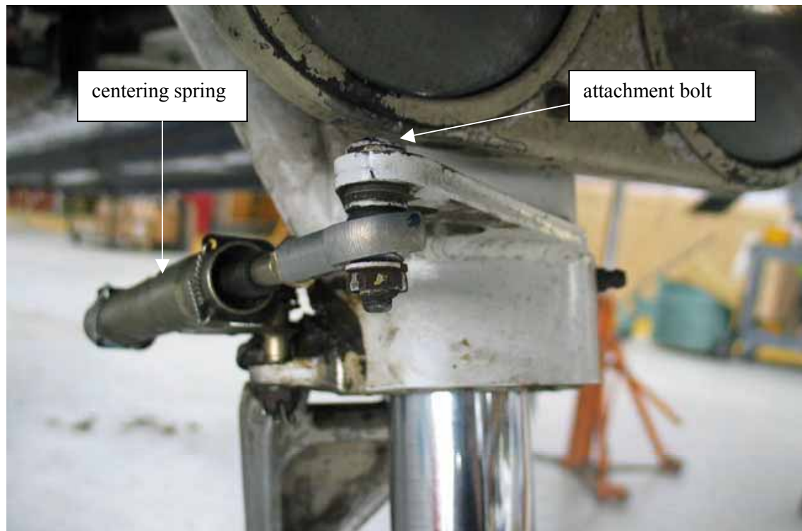
Figure 3 Attachment bolt, incorrectly installed with head up (gear extended)
