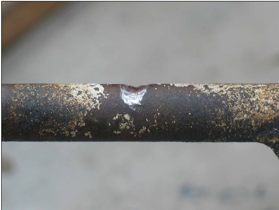
Figure 4 Wear in aft tube assembly
