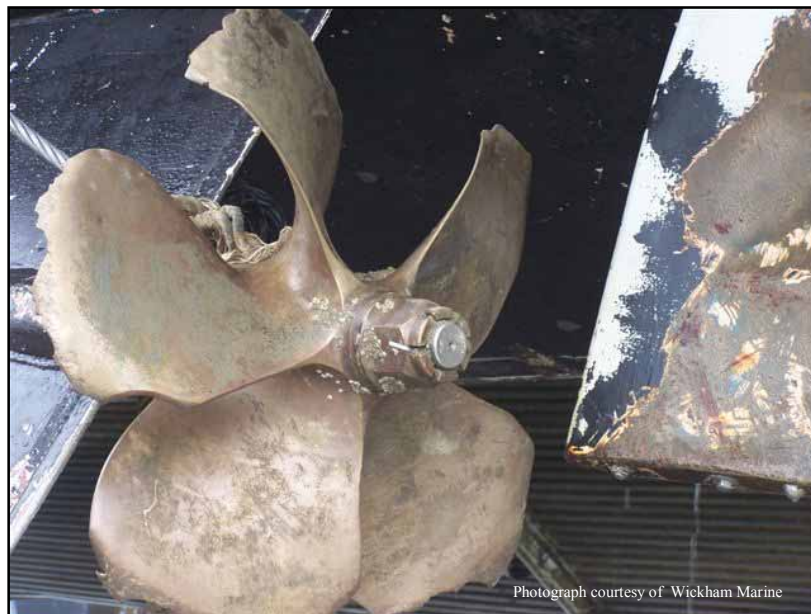
Figure 7 The port propeller showing severe damage to every blade
