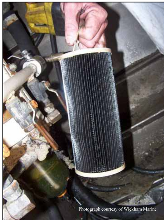
Figure 4 Filter cartridge from the port inboard Racor primary fuel filter
