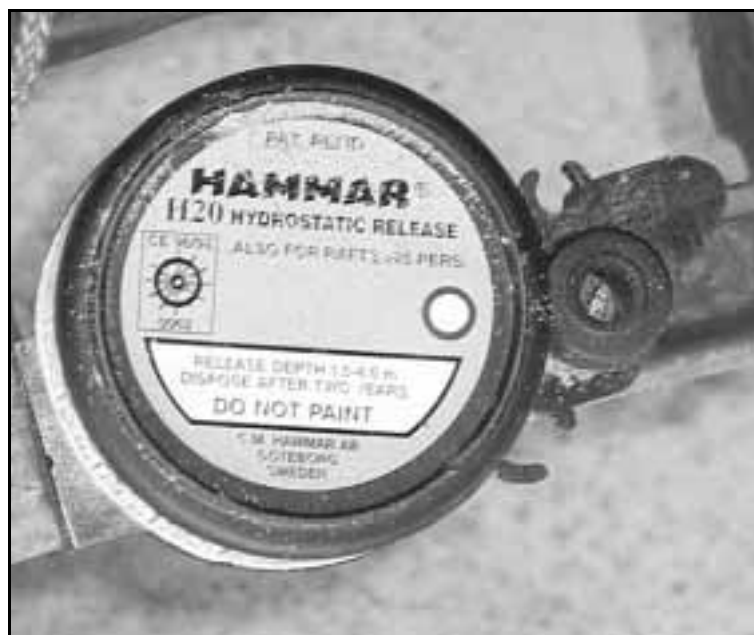
Figure 17 Hydrostatic release found on Twilight Beach
