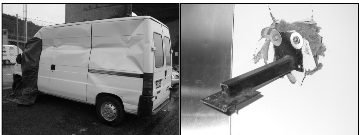
Figure 4 Damage sustained to one cargo van and to the games machines upper retaining arm
