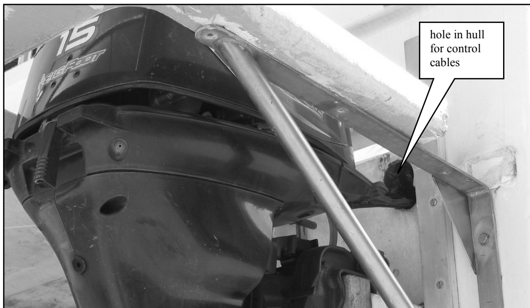
Figure 6 Control cables passing through a hole in the transom
