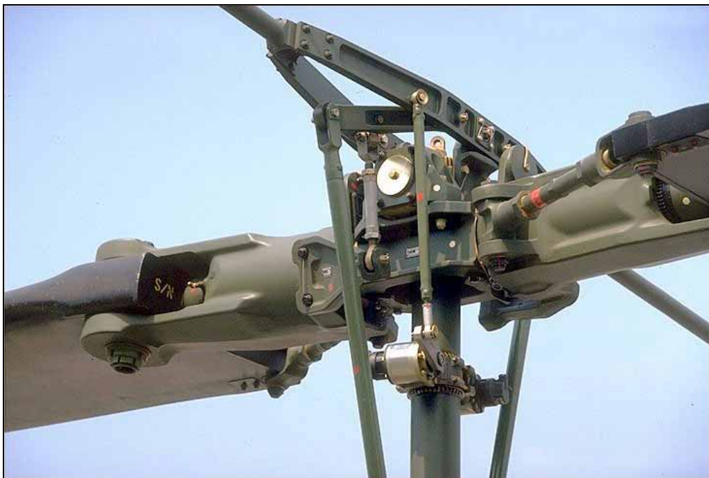
Figure 1 UH-1B main rotor head
