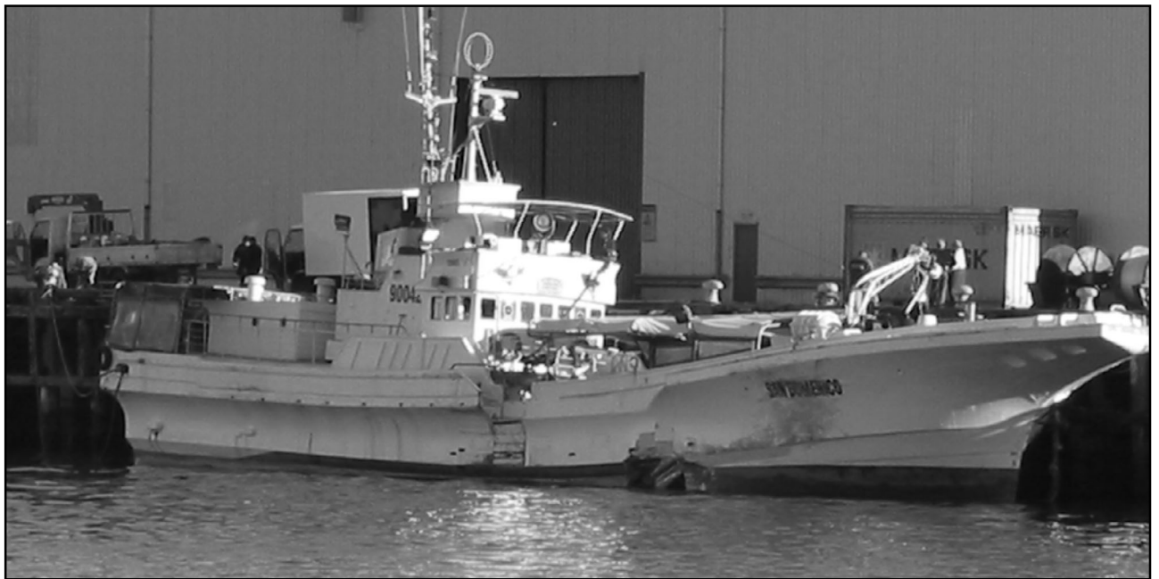
The San Domenico alongside Aotea Quay after the collision, damage visible on starboard side
