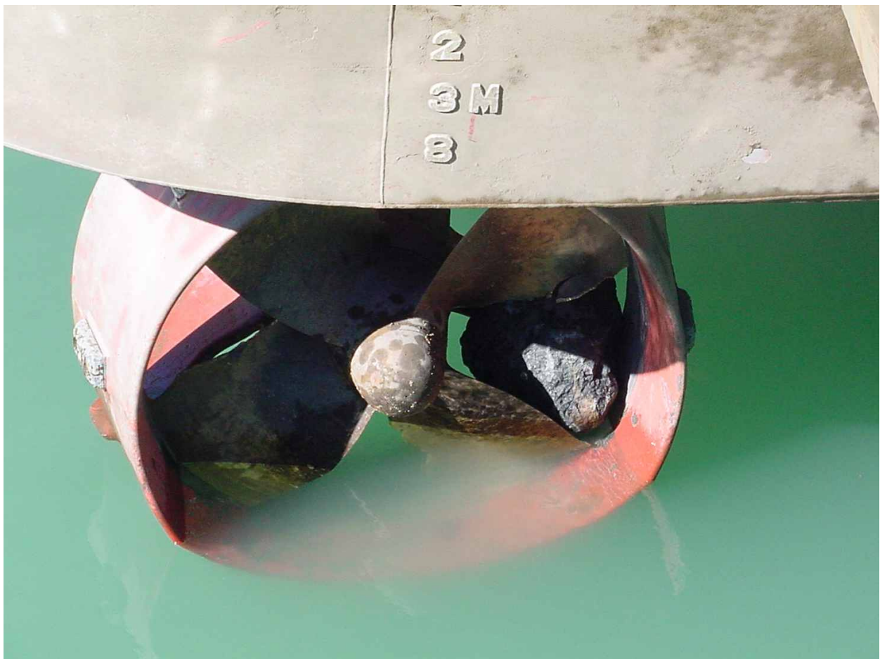
Figure 3 Starboard unit showing the rock jammed in the propeller
