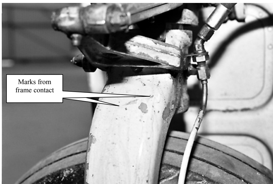
Figure 5 Right lower leg, showing matching marks from frame contact
