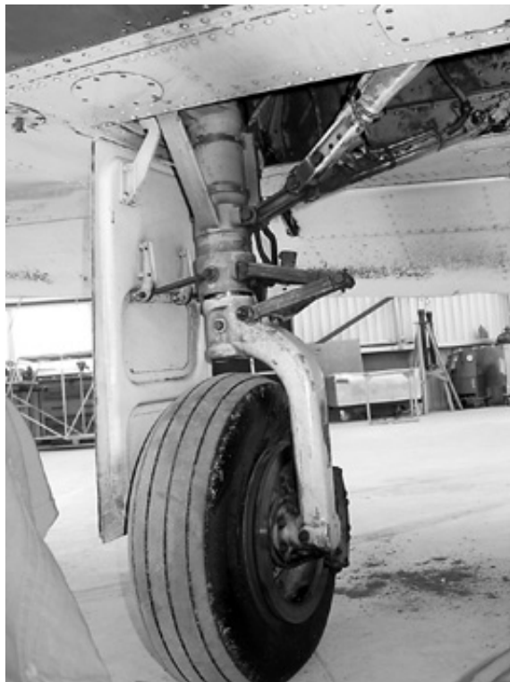
Figure 2 Right undercarriage, showing flat oleo strut
