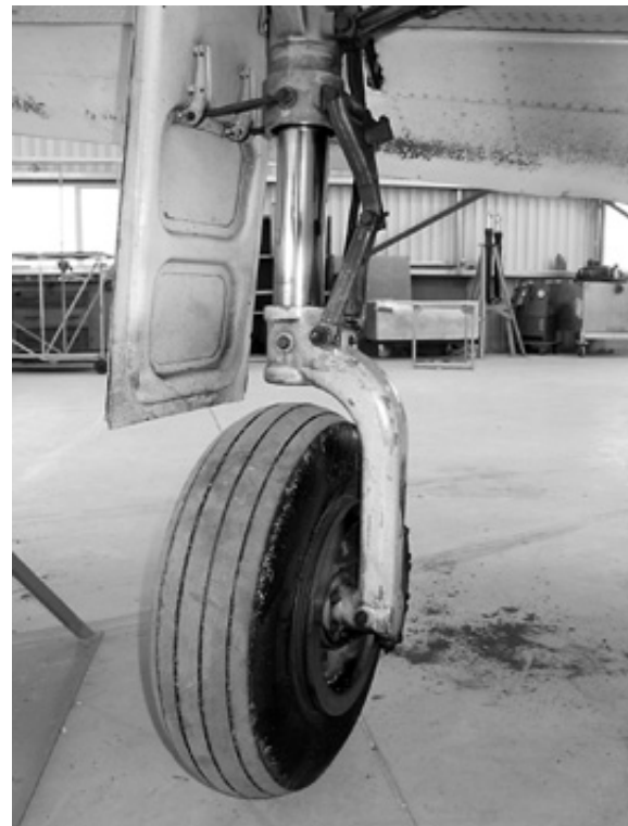
Figure 3 Right undercarriage, oleo strut extended
