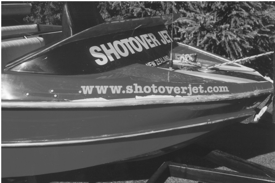
Figure 2 Damage to the starboard bow of Shotover 6
