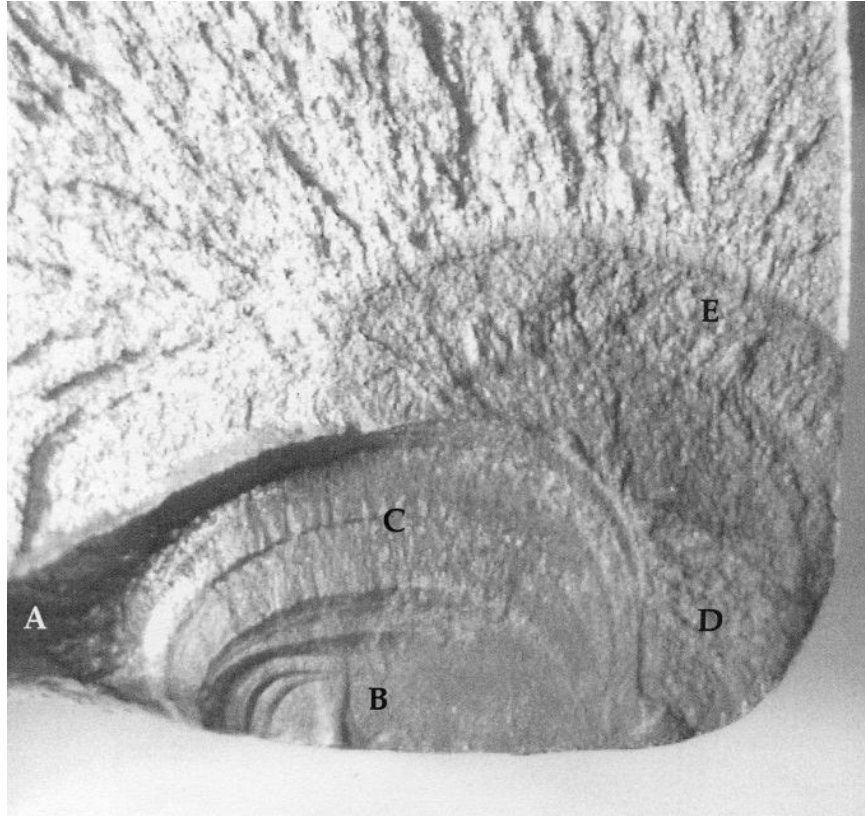
Figure 4 The surface of the fractured wheel showing the 5 cracks
