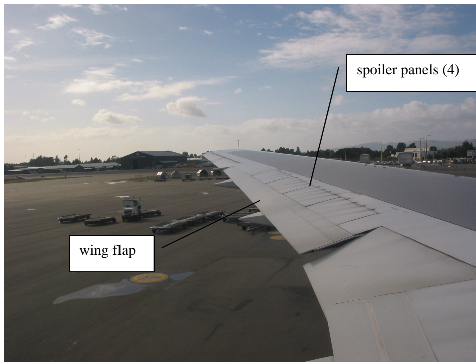
Figure 1 View from row 26 of left wing of Boeing 767-319 (same model as ZK-NCH)
