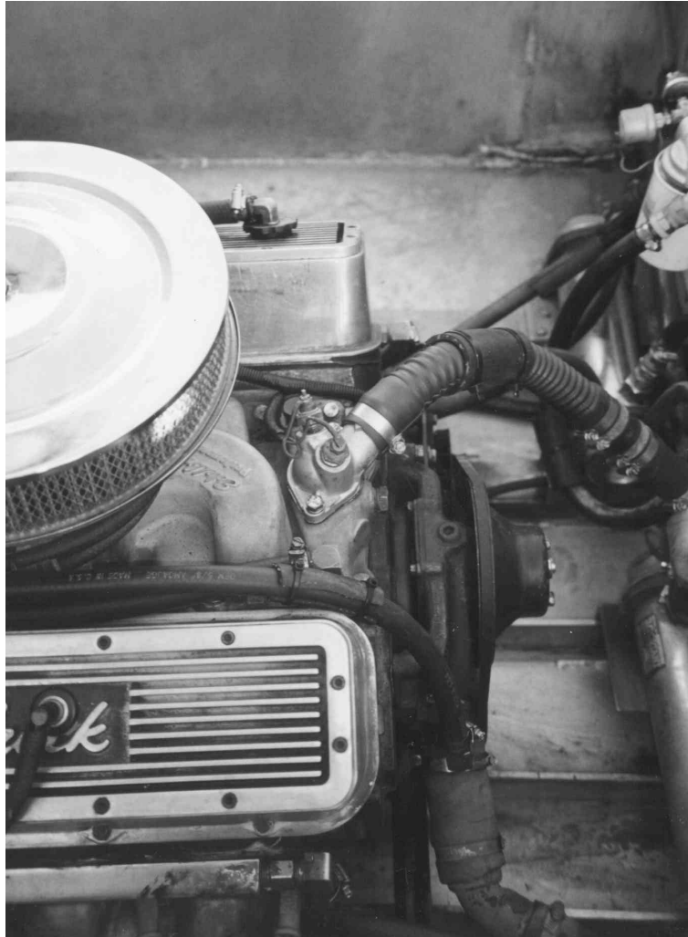
Figure 6 Thermostat housing and associated plumbing
