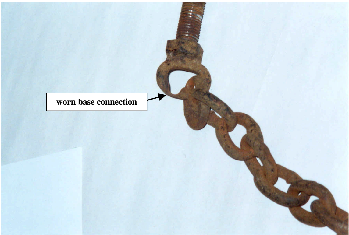
Figure 4 Worn connections from a safety chain under the leading bogie brake rod
