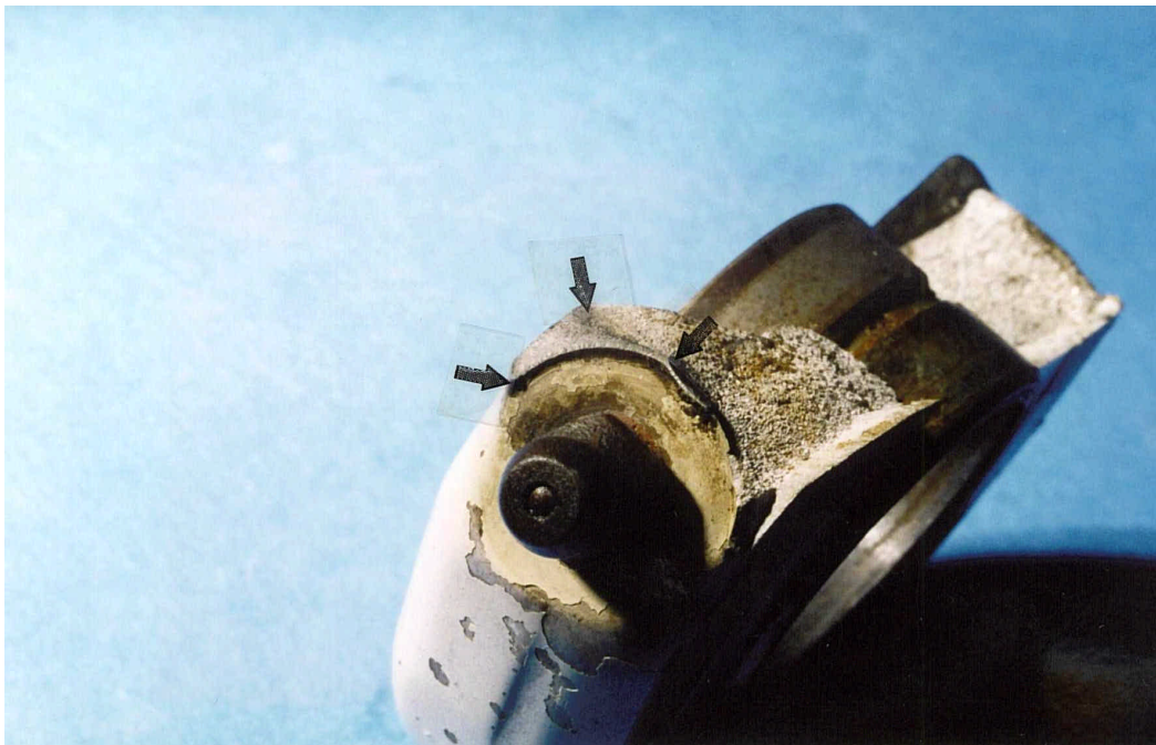
Figure 2 The broken outboard drag brace end piece from ZK-RCA showing the fatigue crack (arrowed)
