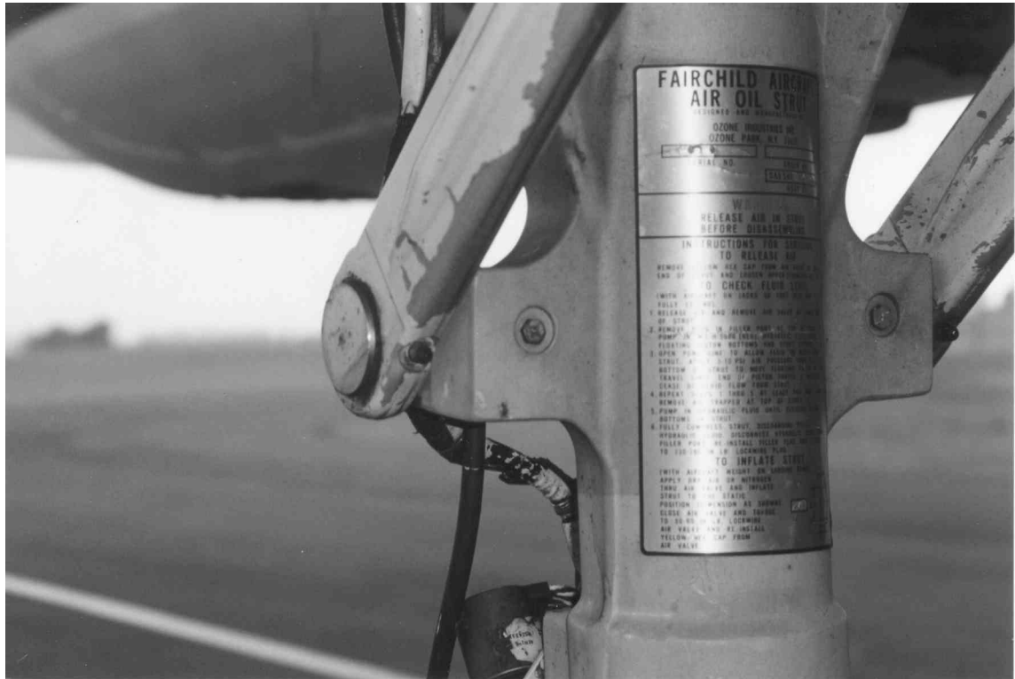
Figure 1 Metro undercarriage leg showing inboard and outboard lower drag braces
