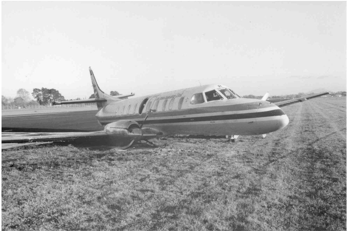
ZK-RCA Metro III After the wheels-up landing
