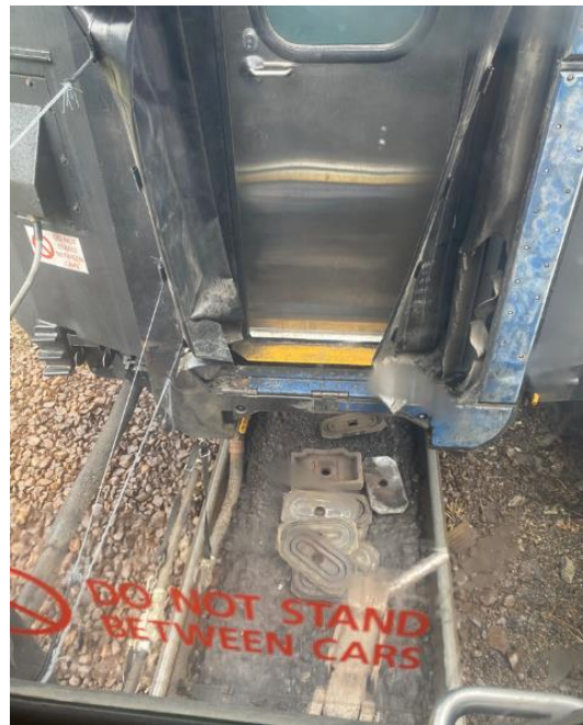
Figure 11 from the report: Parted gap between first and second carriages
