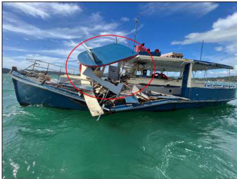
Figure 6 from the report: The damaged Waitere showing the destroyed wheelhouse (Credit: Bay of Islands Coastguard)
